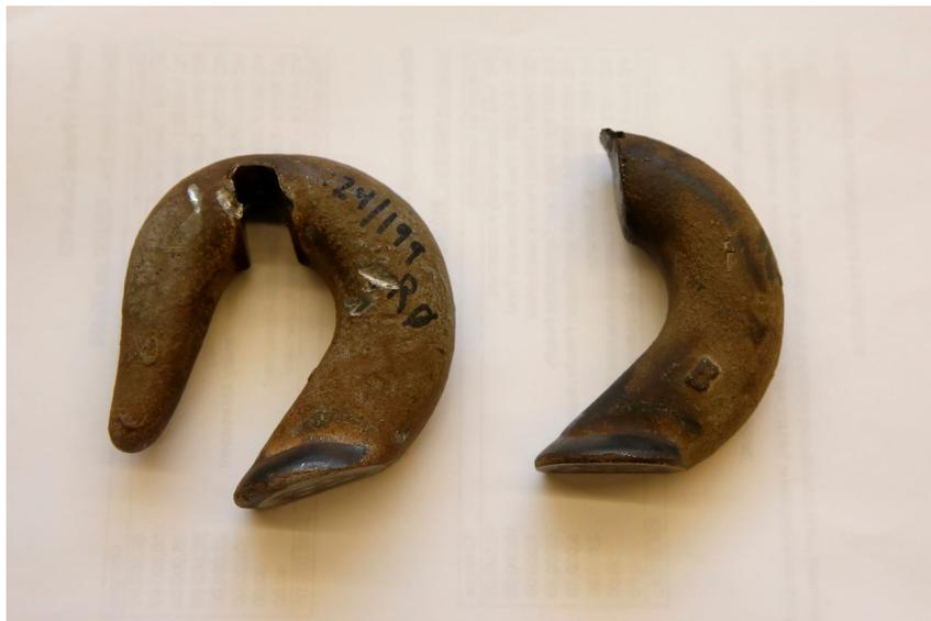
At right, a broken PG&E C hook that investigators determined led to the 2018 Camp Fire. At left, a damaged but unbroken hook.
