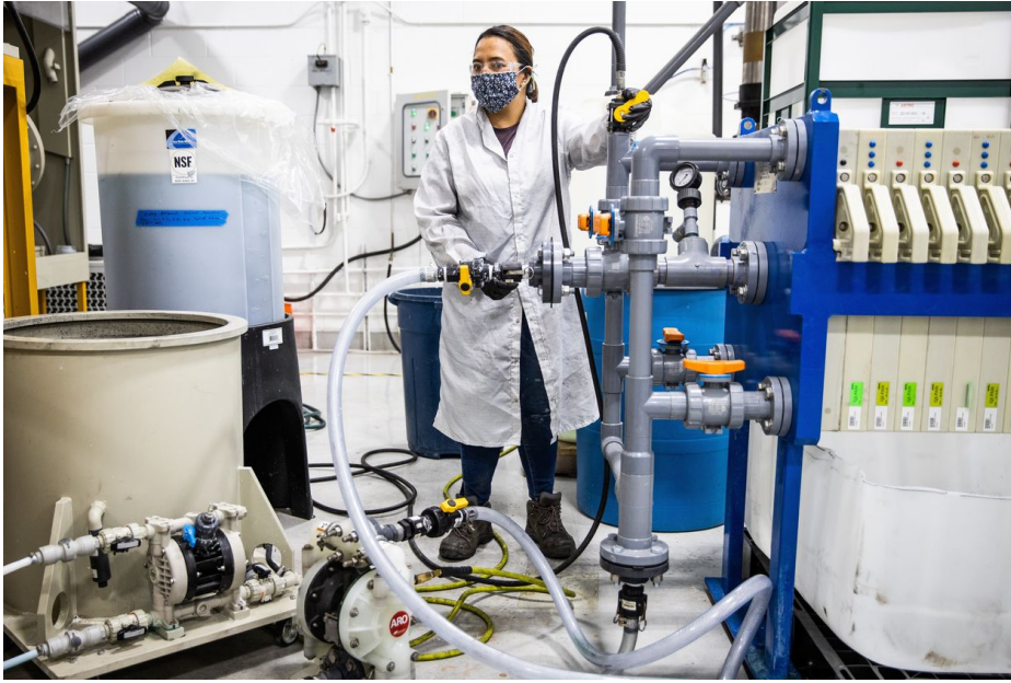
Chemical engineer Fredy Bridges filters metal salts at the Redwood Materials facility in Carson City.
